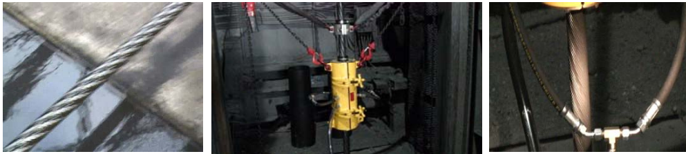
Slope Rope & Personnel Hoist
