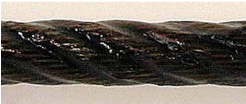
Figure 3. Grease Lubed Wire Rope
