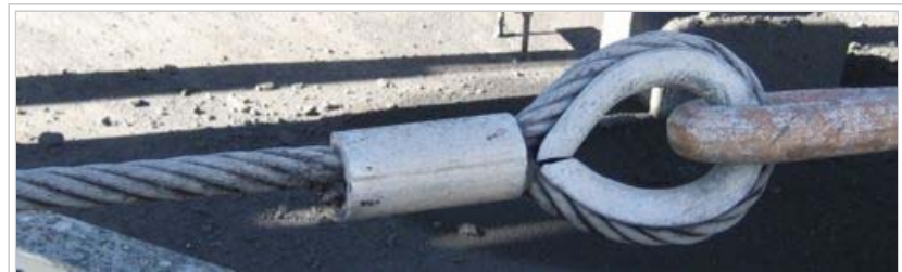
Right-hand ordinary lay (RHOL) wire rope terminated in a loop with a thimble and Talurit brand swaged sleeve.
