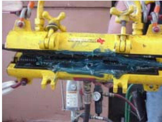
Inside view of lubrication collar, the point where wire rope runs through the automated wire rope lubrication system
