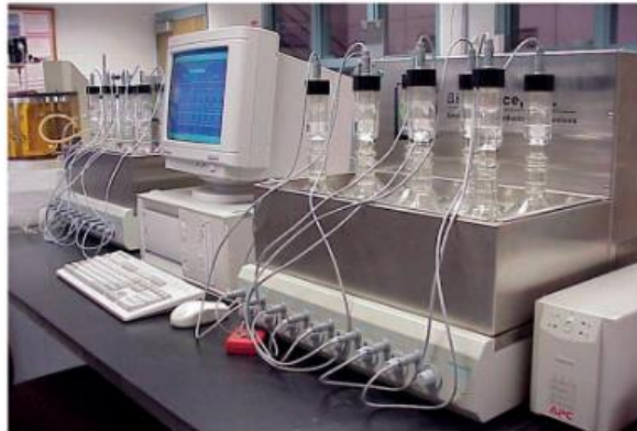
Figure 2. Biodegradability test instrument showing chambers in two separate water baths (Source: Environmental Lubricants Manufacturing Inc.).
