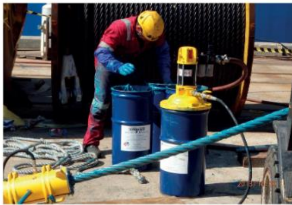
Figure 4. A lubricant applicator uses a drum pump to apply biobased grease to a fast moving wire rope via a lubricant disperser (Source: The Kirkpatrick Group, Inc.).
