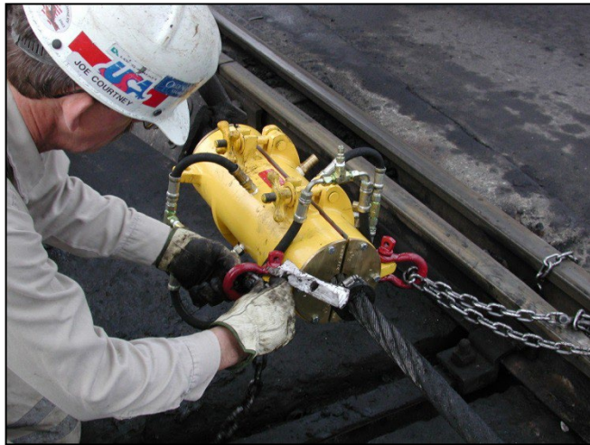
Dynagard LVL Being Applied to a Mine's Slope Rope. Model JU16L, Highland Mining, Kentucky USA
